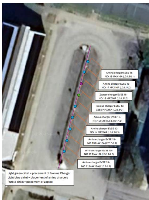
Figure 3 Cluster layout slow charging demonstration.
