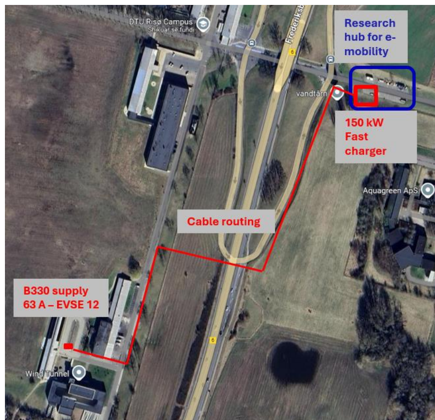
Figure 5 Cable routing for the grid connection of the fast charging demo site.
